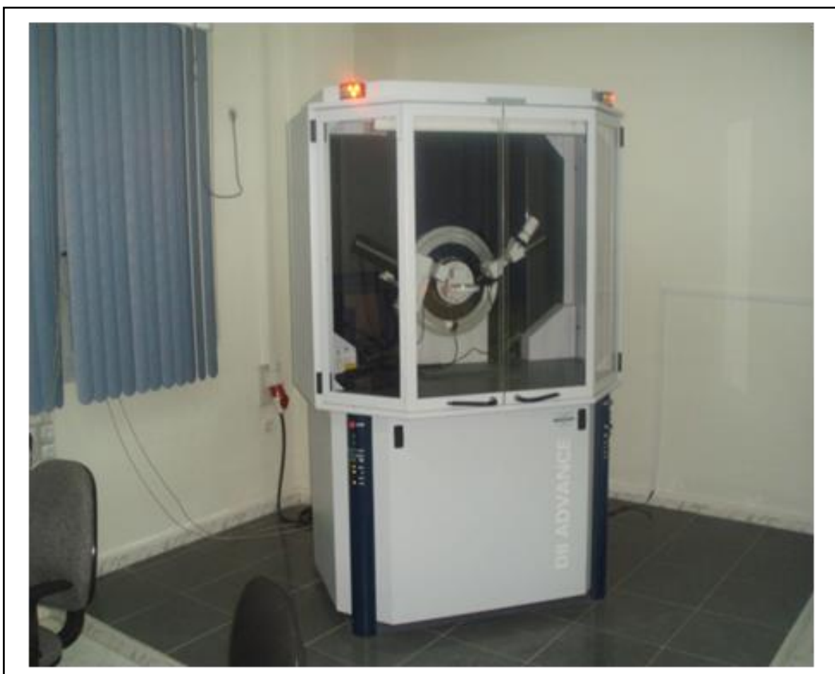
Figure II-7 : Diffractomètre Panalytical X'Pert (D8 ADVANCE) BRUKER.
