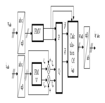
Figure. 2: The method of instantaneous active and reactive power
