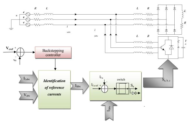
Figure.1 -Network and shunt active filter presentation
