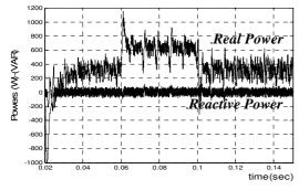
Fig. 10. Input real and reactive powers.
