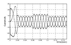
Fig.11. Stator currents.
