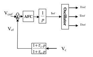
Fig. 5. Block diagram of adaptive fuzzy voltage control.
