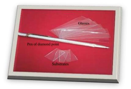
Fig.II.1. The used Glasses substrates and diamond pen.
