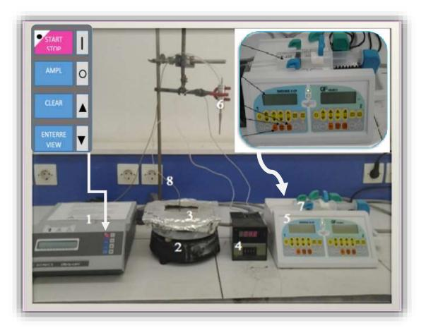
FigII.2. ultrasonic spray technique setup that used.
