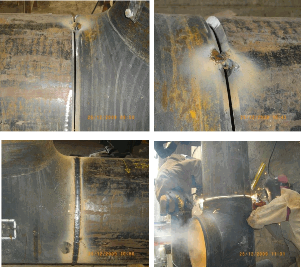
Figure. III.3 : Steps of the weld joint preparation.
