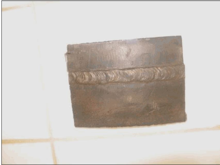
Figure III.4: Sample (30x20 cm) of the welded pipe line.
