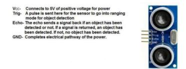
Figure 25: Ultrasonic Sensor HC SR-04
