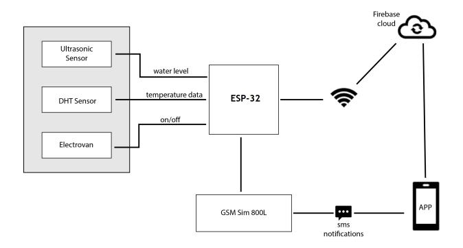
Figure 30: System Block Diagram
