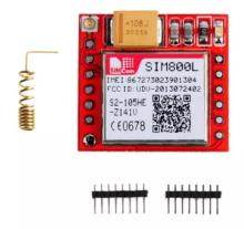
Figure 23: SIM-800L GSM Module
