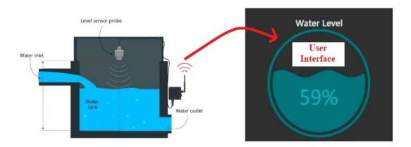
Figure 3: The Functionality of the smart water level monitoring system
