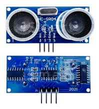
Figure 9: Ultrasonic sensor (HC SR-04)
