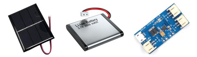
Figure 28: Solar Charging System
