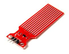
Figure 8: Water depth sensor
