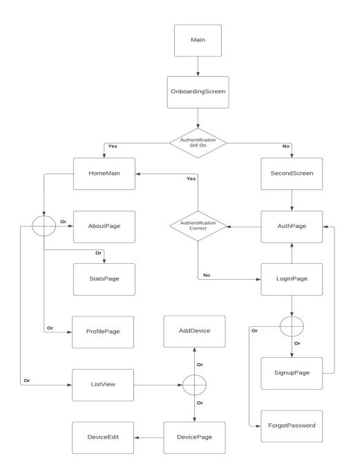
Figure 36: Flowchart of the mobile application
