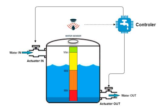
Figure 2: Smart water tank schema with sensors to monitor and control water valves
