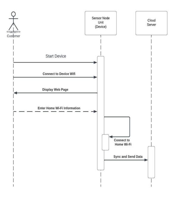
Figure 34: Sequence diagram of the configuration
