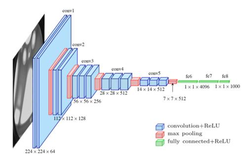
Figure 1.24: The standard VGG16 network architecture diagram[32].
