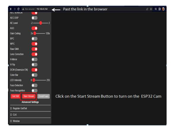
Figure 3.13: Past the link and turn on the ESP32 camera.
