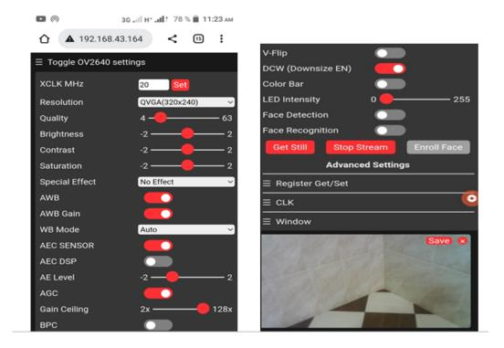
Figure 3.15: Control ESP32 camera from Mobile phone
