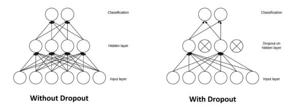
Figure 1.19: Example of dropout[4].
