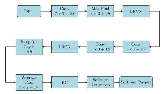
Figure 1.23: A simplified block diagram of the GoogLeNet Architecture[32].
