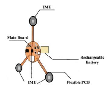
Figure 3.7: The Wearable Design Proposed to Monitor Fetal Movements Alim and Imtiaz (2023)
