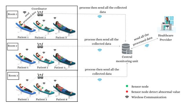
Figure 3.11: Decentralized Data Processing in the Third Scenario
