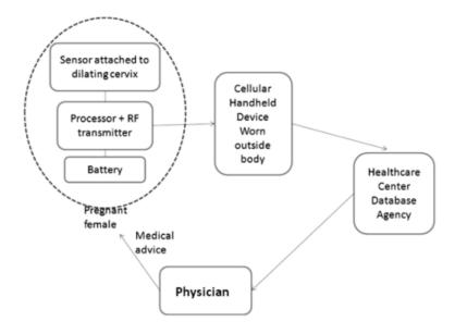
Figure 3.6: A Schematic Diagram for Monitoring Cervical Dilation. The arrows represent wireless RF links Verma et al. (2009)
