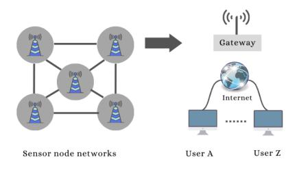
Figure 1.3: Wireless Sensor Network (WSN)
