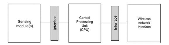
Figure 1.1: The Anatomy of a Sensor Node Bar-Noy et al. (2005)
