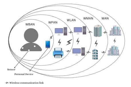
Figure 1.5: Positioning of a Wireless Body Area Network in the Realm of Wireless Networks
