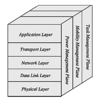
Figure 1.4: WSN Architecture A. A. A. Alkhatib and Baicher (2012)
