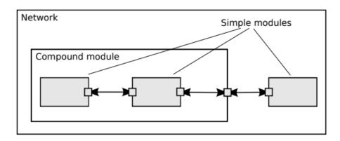
Figure 4.1: Simple and Compound Modules Varga (2019)
