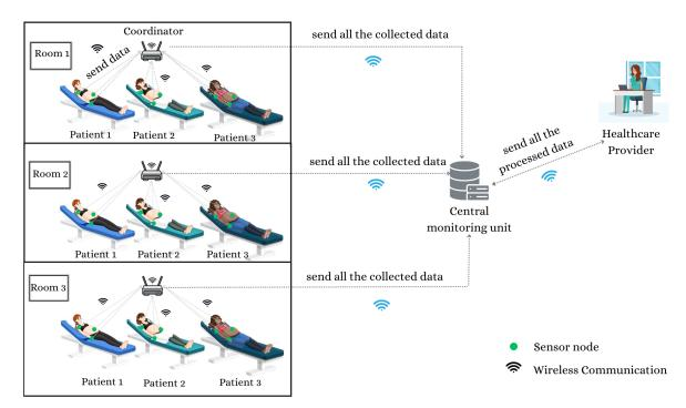
Figure 3.9: Centralized Data Processing in the First Scenario
