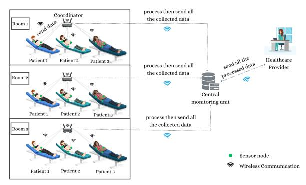
Figure 3.10: Semi-Centralized Data Processing in the Second Scenario
