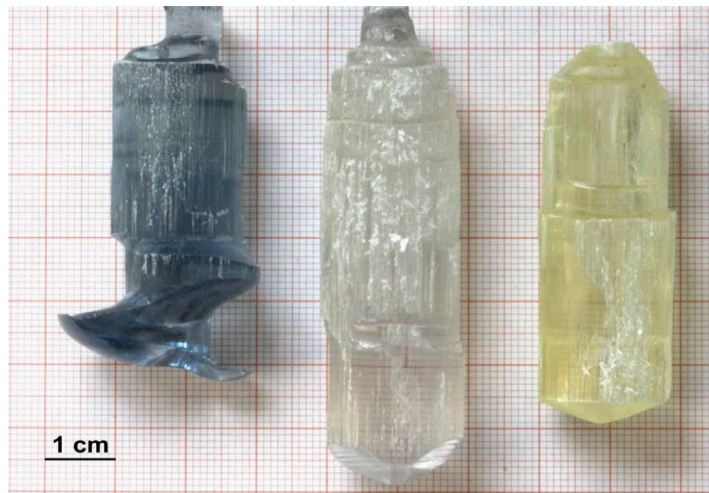
Figure I.17: Some examples of coloration of \beta\text{-Ga}_2\text{O}_3 crystals[33].
