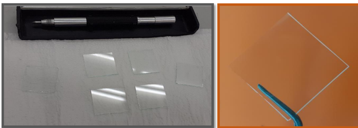
Fig.III.1 Glass substrates and diamond-tipped pen.
