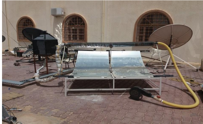
Figure III-5 Solar dryers with cylindrical-parabolic collector
