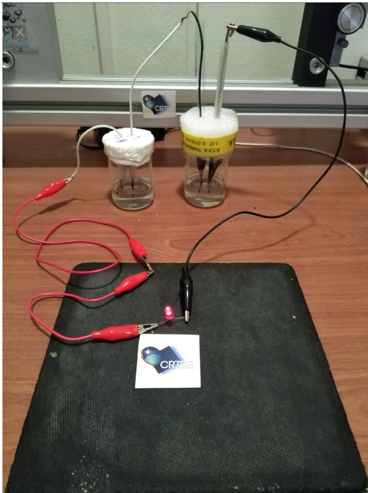
Fig. IV. 28. Photograph of a red LED eliminated with two cells serially connected.
