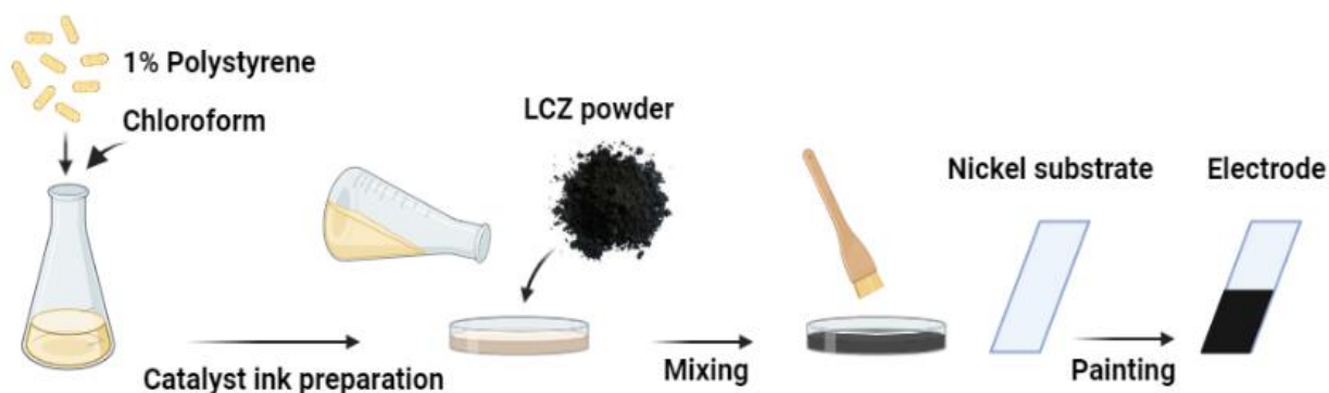
Fig. III. 2. Schematic of LCZ electrodes preparation steps.
