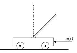
Fig. 1. The inverted pendulum system
