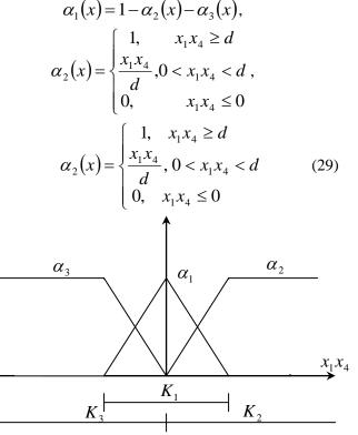
Fig. 2, Membership functions and local controllers
