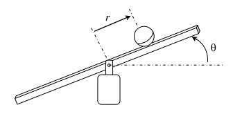
Fig. 1 Ball and beam system
