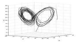
Fig. 1. The phase trajectory of the controlled Lorenz system.
