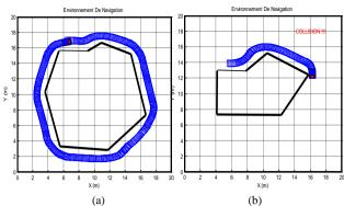
Figure 7. (a) Wall following using fuzzy controller (b) Collision with the obstacles
