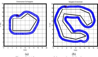
$\label{eq:Figure 8. (a) Improvement of the previous behavior} \end{center} (b) Wall-following with different forms using FQL algorithm$
