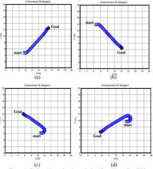
Figure 4. Goal seeking using the optimized fuzzy controller (FQL)
