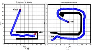
Figure 11. Navigation in a Corridor Figure 12. Wall-following
