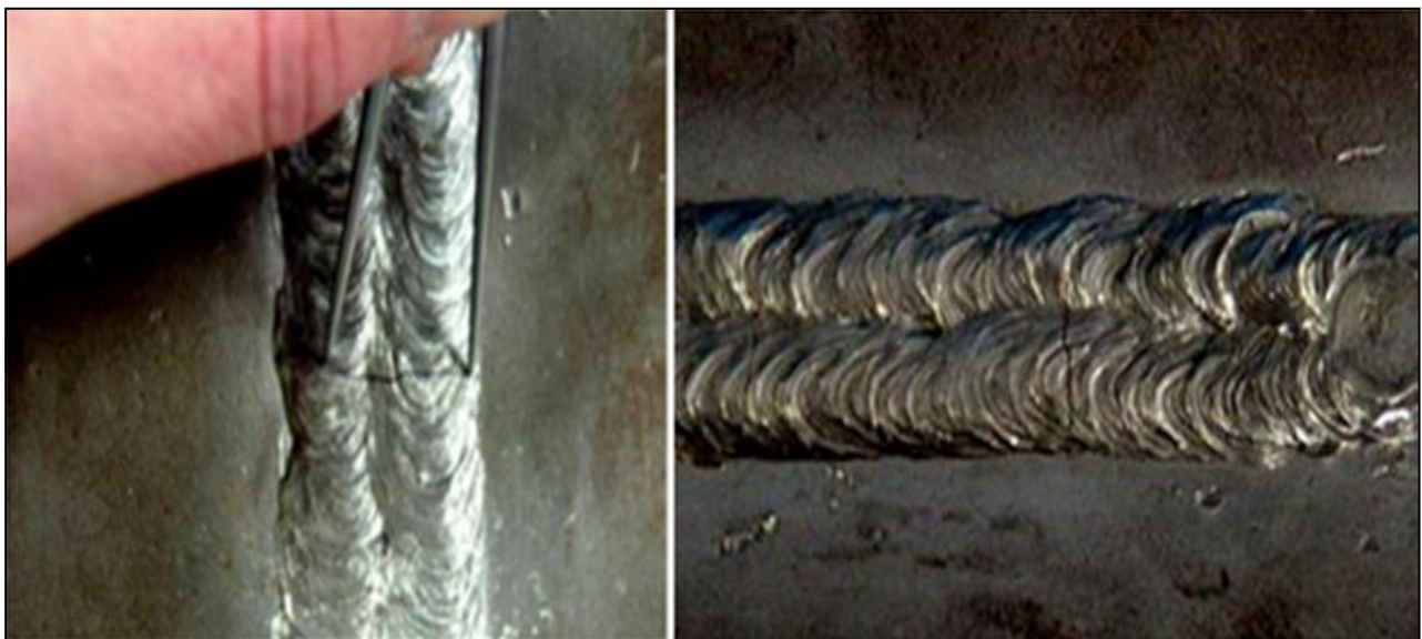
Figure 10 b : La fissure transversale.
