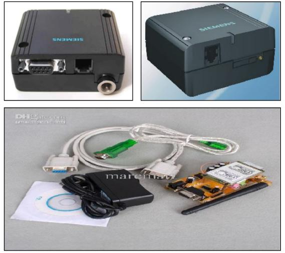
FigII.1. TC35 GSM module and its components.[12]
