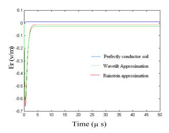
Figure 9: The horizontal electric field variation using the TL modelr = 12 km, z = 6 m.
