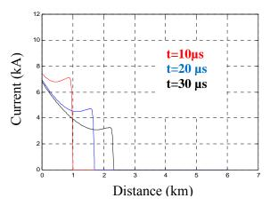
Figure 3: Spatial current distribution along the lightning channel.
