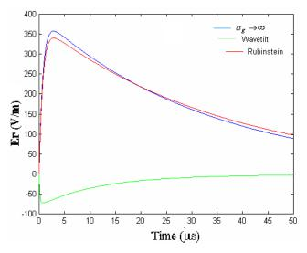
Figure 6: The horizental electric field variation using the TL modelfor r= 200m, z=10m
