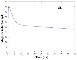
Figure 4: The magnetic field at 50 m from a lightning return stroke obtained by the proposed method [7]
