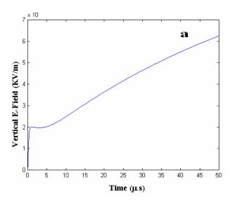
Figure 5: The electric field at 50 m from a lightning return stroke obtained by the proposed method [7].
