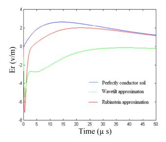
Figure 8: The horizontal electric field variation using the TL modelr = 1.5 km, z = 100 m.
