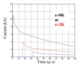
Figure 2: Temporal current distribution along the lightning channel
