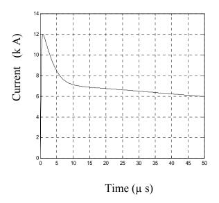
Figure 1: Time-variation of the channel- base current.
