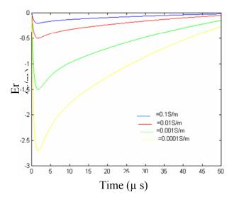
Figure 10: The horizontal electric field variation using the TL model for different conductivity with the use of Wavetilt approximation. r = 2 km, z = 6 m.
