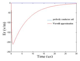
Figure 7: The horizental electric field variation using the TL modelat 100 m from lightning
