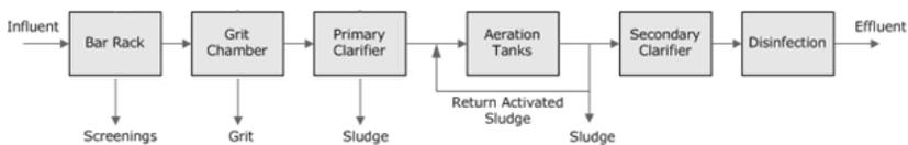
**Figure 2:** Process scheme of Batna WWTP.
