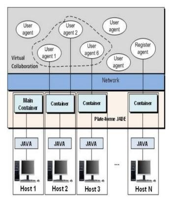
Figure 5: Implementation of architecture using JADE.
