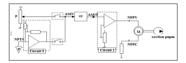
Figure III.12. Simplified Electrical Circuit Pressure
