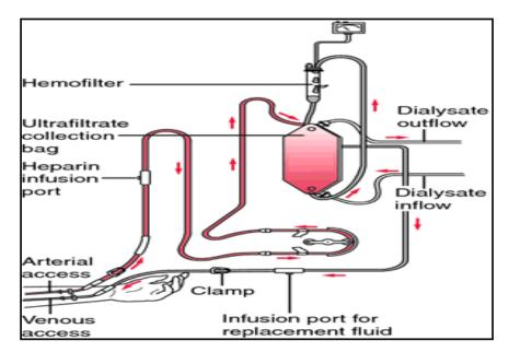
Figure II.4. A hemodialysis circuit
