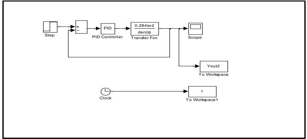
Figure.III.18. Simulink model with PID
