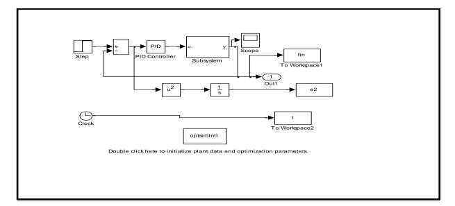
Figure III.20.Simulink Model with ABC-PID
