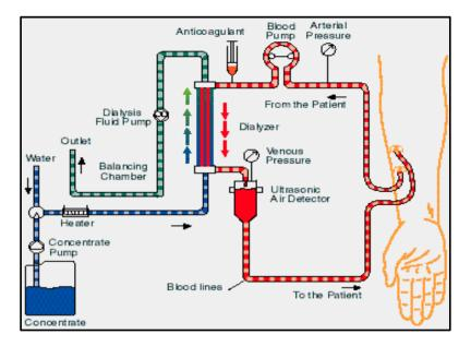
Figure II.3. Principle of hemodialysis
