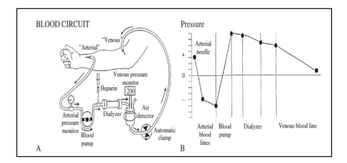
Figure II.5. Operation of an artificial kidney
