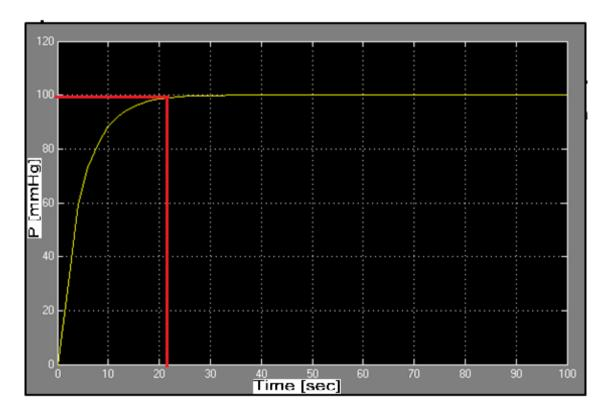
Figure III.21.Response with Proposed ABC-PID
