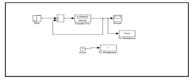
Figure III.16. Simulink Model with Closed Loop
