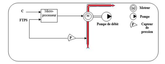
Figure.III.11.Simple Diagram of the Pressure Control Loop
