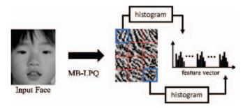
Fig. 1: Example of MB-LPQ features extraction with  $4 \times 3$  sub-blocks.
