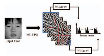
Fig. 2: Example of ML-LPQ features extraction with 4 level.
