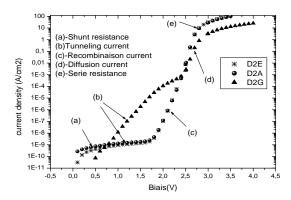
Figure 2: Measured forward characteristics of 4H-SiC of 3 diodes at 298K.
