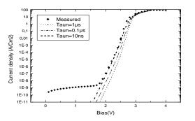
Figure 3: Measured and simulated forward characteristics of diodes D2A at 298K for variouscarriers'lifetimes.
