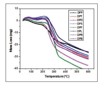
**Figure 7.** Thermogravimetric curves of date palm wood: (DPP)Petiole, (DPT)Thorns, (DPD)Pedicels, (DPS)Spathe, (DPF)Fibrillium, (DPL)Leaflets, (DPR)Rachis, (DPB)Bunch.
