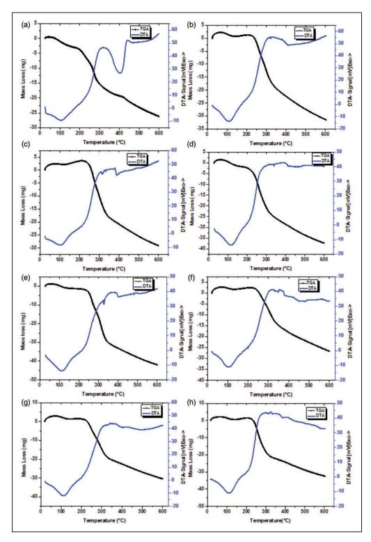
Figure 6. Thermal analysis of date palm wood: (a) Petiole, (b) Thorns, (c) Pedicels, (d) Spathe, (e) Fibrillium, (f) Leaflets, (g) Rachis, (h) Bunch.
