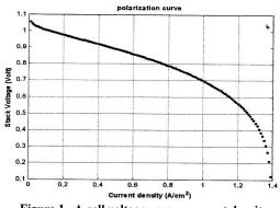
Figure 1. A cell voltage versus current density
