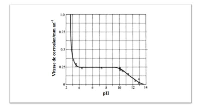
Figure I-10: Change in the corrosion rate of the steel on function of pH.
