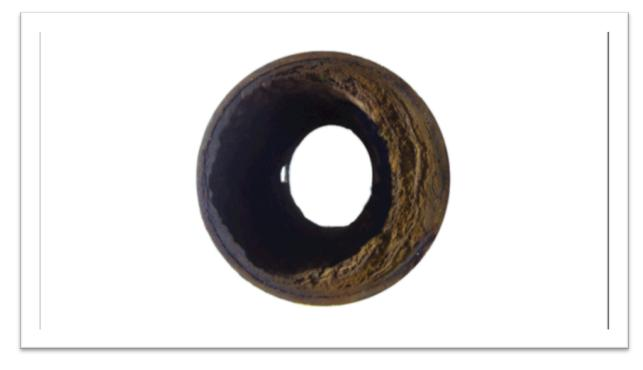
Figure I-1: The cross section of the "scale" of a pipe
