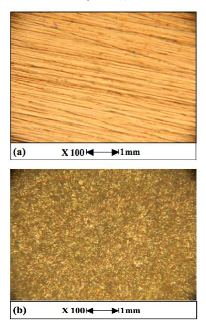
Figure III-4 : The steel corrosion product morphology API 5L X42 by the optical microscope (x100), (a) the steel without corrosion product, (b) immersing the steel in HCl (116 hours).
