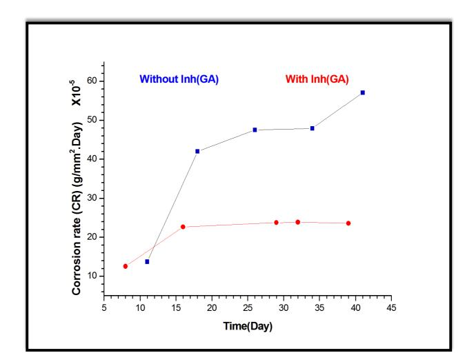
Figure III-1: Relationship between the corrosion rate (CR) and immersion time (Day) with and without GA (2g/l) in 1 M HCl.
