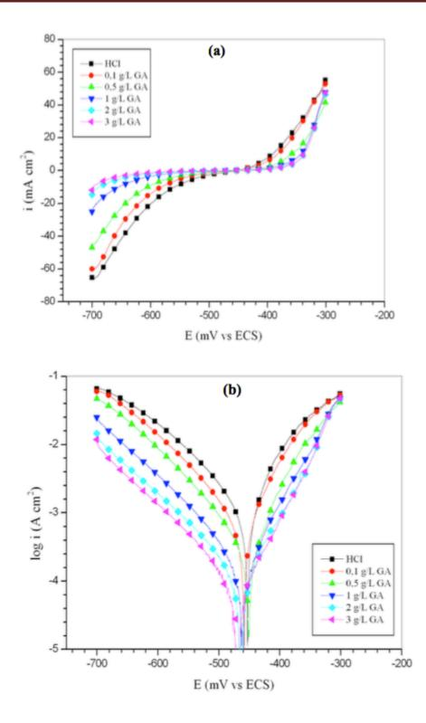
Figure III-17 : Potentiodynamic polarization curves for API 5L X42 pipeline steel in 1 M HCl without and with various concentrations of GA at 35 °C, (a) Linear curve curve,(b) Logarithmic .
