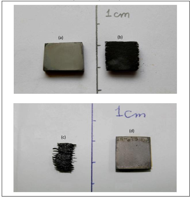
Figure III-13 : Microscopic morphology of API 5L X42 carbon steel after immersion test (264 hours) in HCl medium with 4g/L GA (a), without GA (b). After Immersion test (437 hours) in HCl medium without GA (c), with 4g/L GA (d).
