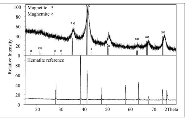
Figure II-10 : XRD of a powder (top) and hematite reference (bottom)
