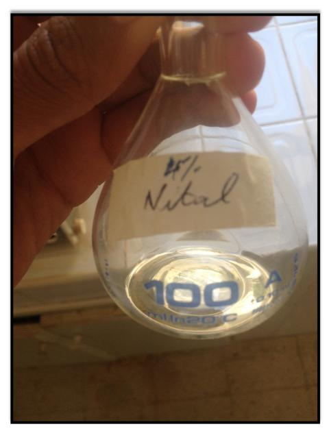
Figure II-4 : Solution of " Nital 4%" used for the attacking process .
