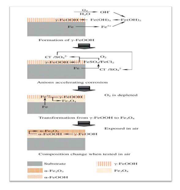
Figure I-9: Evolution of rust layers on carbon steel sample immersed in a simulated solution.
