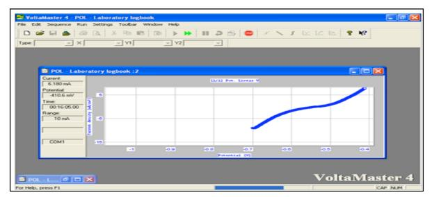
Figure II-8: Polarization curve of API 5L X42 in hydrochloric acid medium 0.1 M (during the test).
