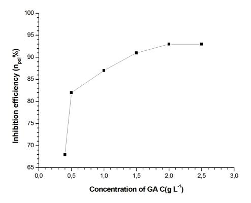
Figure III-16 : Relationship between inhibition efficiency ( $\eta_{pol}$ ) and concentration of GA (g L<sup>-1</sup>) in 1 M HCl at 25 °C(API 5L X42 pipeline).
