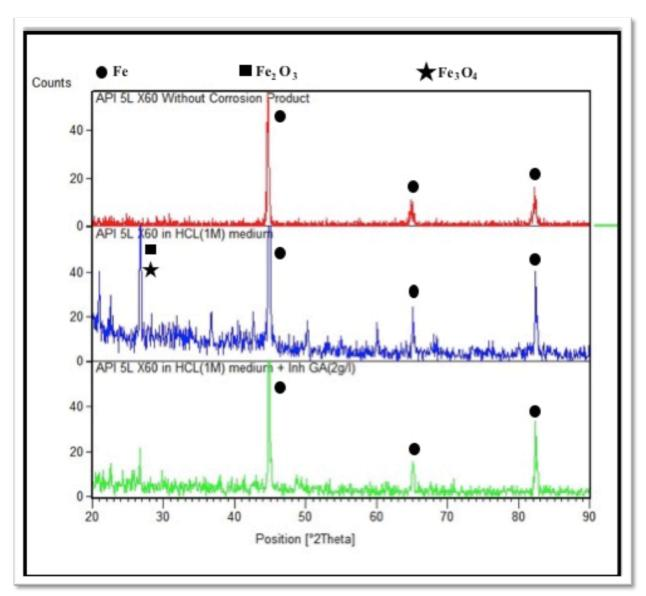
Figure III-10: XRD of API 5L X60 in HCl (648 h) without and with GA (2g/L).
