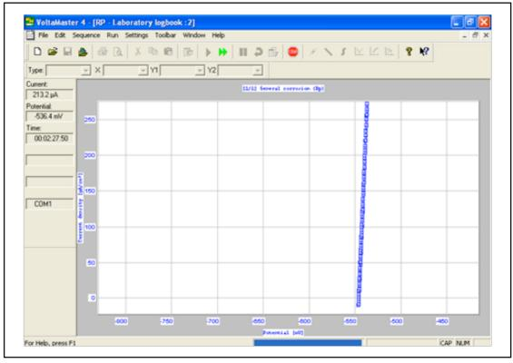
Figure II-1 : Polarization of API 5L (X60 ; X42) in 1M hydrochloric acid medium, in the vicinity of corrosion potential .
