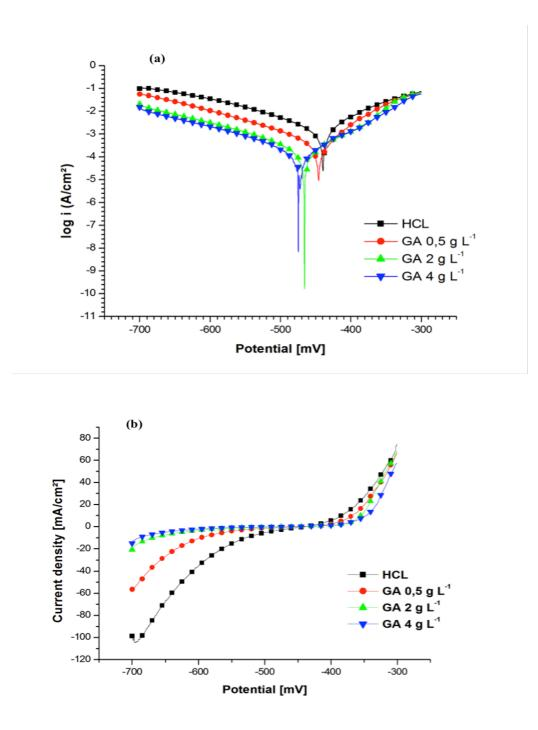
Figure III-15 : Potentiodynamic polarization curves for API 5L X60 pipeline steel in 1 M HCl without and with various concentrations of GA at 45  $^{\circ}$ C, (a) Logarithmic,(b) Linear curve curve. .
