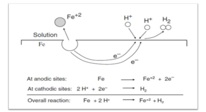
Figure I-2: Coupled electrochemical reactions
