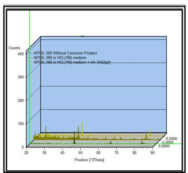
Figure III -11: XRD of API 5L X60 in HCL(648 h) without and with GA(2g/L) in 3D view.
