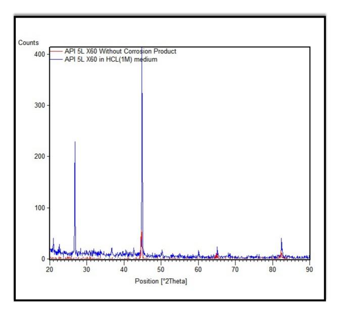
Figure III-3 : XRD of API 5L X60 without corrosion product, with corrosion product in HCl medium (648 h).
