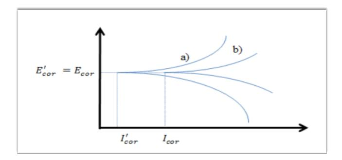
Figure I-16 : Theoretical potentiostatic polarization diagram: electrochemical behavior a metal on a solution containing a cathodic and anodic inhibitor (a) compared to the same solution without the inhibitor (b).
