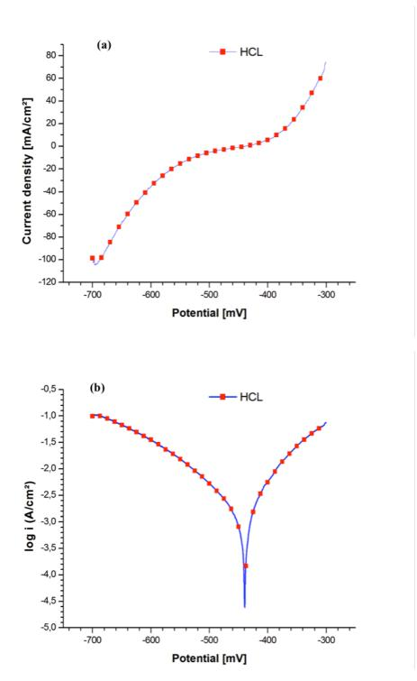
Figure III-7: Cyclic voltammetry of API 5L X60 in HCl medium at 45 ° C, (a) Linear curve, (b) Logarithmic curve.
