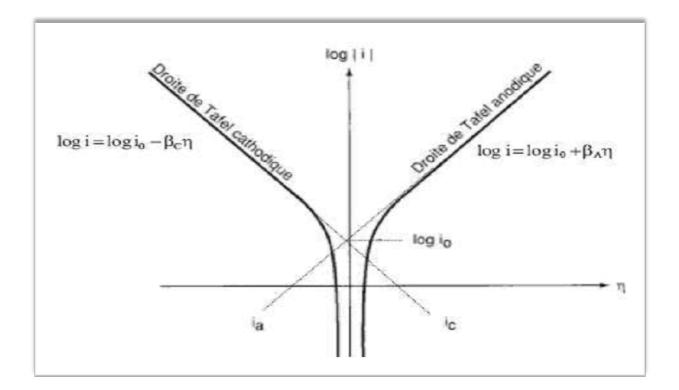
Figure I-4: Polarization curves and Tafel line(s).
