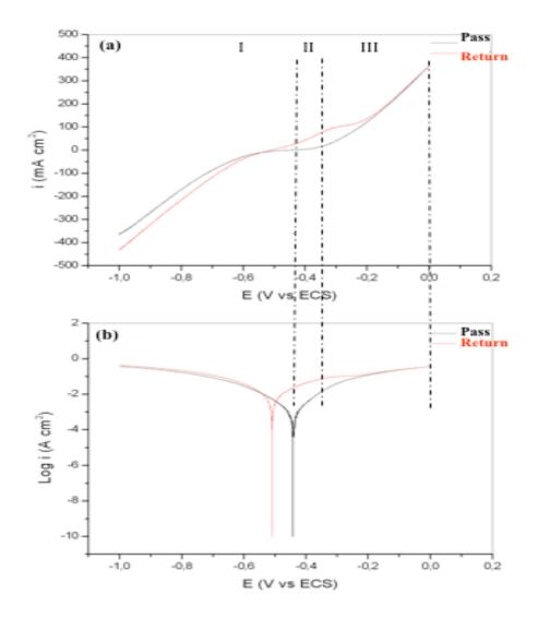
Figure III-5: Cyclic voltammetry of API 5L X42 in HCl medium, (a) Linear curve, (b) Logarithmic curve.
