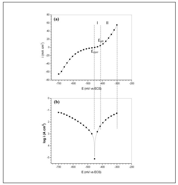
Figure III-6:Polarization curves of API 5L X42 in HCl medium at 35 ° C, (a) linear curve, (b) logarithmic curve.
