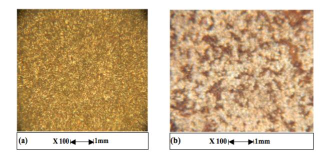
Figure III-9: The morphology of API 5L X42 corrosion products by the optical microscope (x100), (a) immersing the carbon steel in HCl (116 hours) without GA, (B) immersing the carbon steel in HCl (116 hours) with 4g / L GA.
