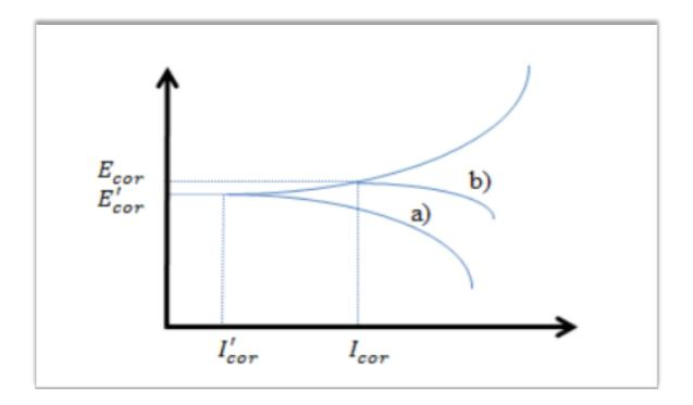
Figure I-14 : Potentiostatic polarization diagram: electrochemical behavior of the metal in a cathodic inhibitors solution (a), as compared to the same solution, without inhibitor (b).
