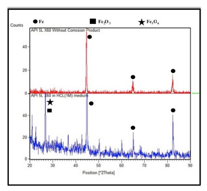
Figure III-2 : XRD of API 5L X60 without corrosion product, with corrosion product in HCl medium (648 h) in 2D view.
