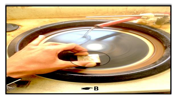
Figure II-2 : Photographs of the apparatus used. A: Polisher ; B :Sample polished on abrasive disc
