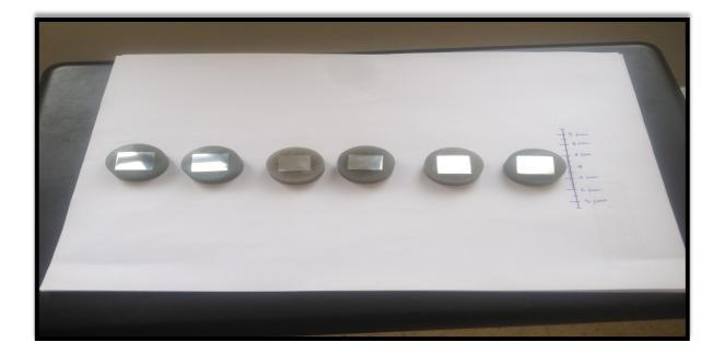
Figure II-3 : Appearance of API 5L X60 samples with resin coating before the immersion test.
