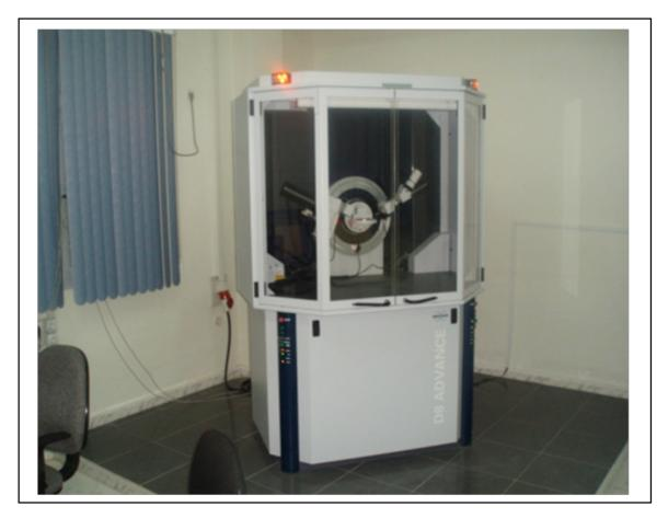
Figure II-9 : X'Pert diffractometer Panalytical (D8 ADVANCE) BRUKER.
