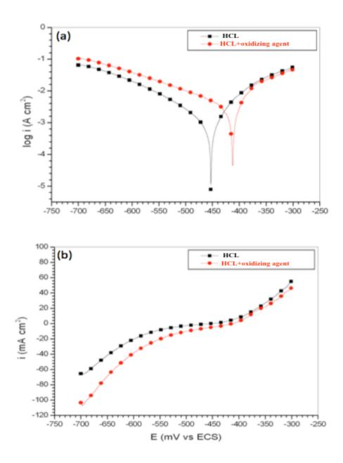
Figure III-8 : logarithmic polarization curves (a) ; linear (b) of API 5L X42 steel in 1M HCl medium without and with  $Fe^{3+}$  at 35 ° C.
