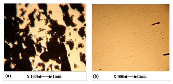
Figure III-12: Photography by the optical microscope shows the effectiveness of GA after the immersion test. (a) HCl medium without GA (264 hours), (b) HCl medium with GA (264 hours).
