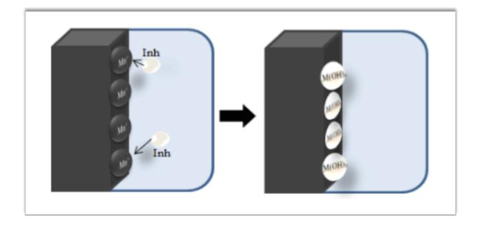
Figure I-15 : Illustration has shown the mechanism of actuation of the cathodic inhibitors.
