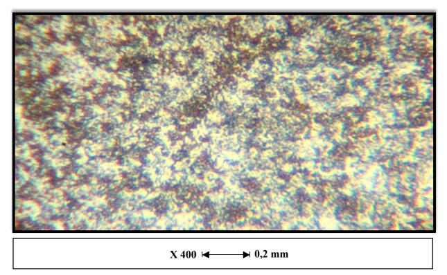
Figure II-6 : Metallographic structure of carbon steel API 5L X42 performed after an attack by nital 4%.
