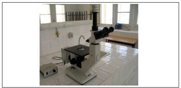
Figure II-11 : Optical microscope HUND T100-WETZLAR
