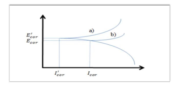
Figure I-12 : Potentiostatic polarization diagram: electrochemical behavior of a metal in a solution with anodic inhibitor (a) *versus* without inhibitor (b).
