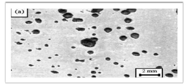
Figure I-8: Localized corrosion (Pitting) morphological view after pitting corrosion of steel in a chloride medium.
