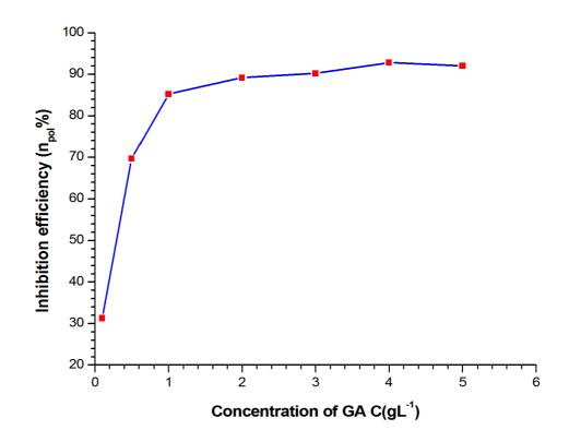
Figure III-14 : Relationship between inhibition efficiency ( $\eta_{pol}$ ) and concentration of GA (g L<sup>-1</sup>) in 1 M HCl at 45 °C (API 5L X60 pipeline).
