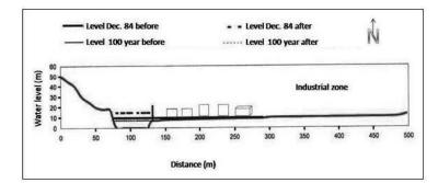
Figure 10: The Effect of dyke construction on flood levels in the industrial zone of Skikda
