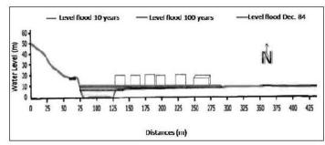
Figure 7: Wadi Saf-Saf in vicinity of the industrial zone: Cross section and levels of the probable peak flows
